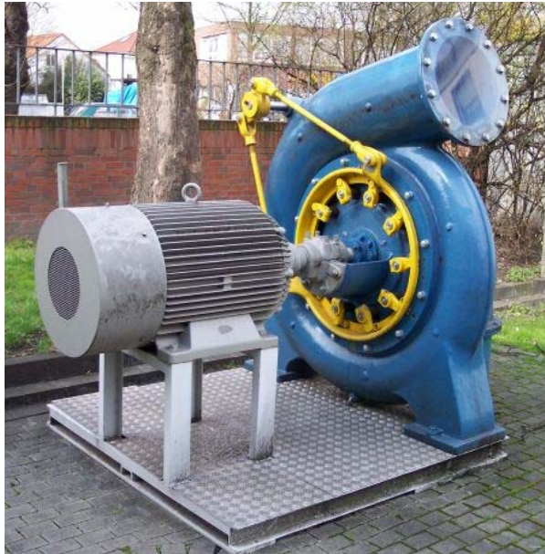
Figure 8.5 Francis Turbine connected to generator (Wikipedia, 2006)
