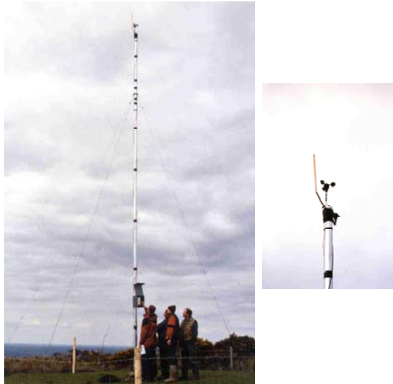
Figure 7.10 Anemometer (Tipperary Institute, 2006)
