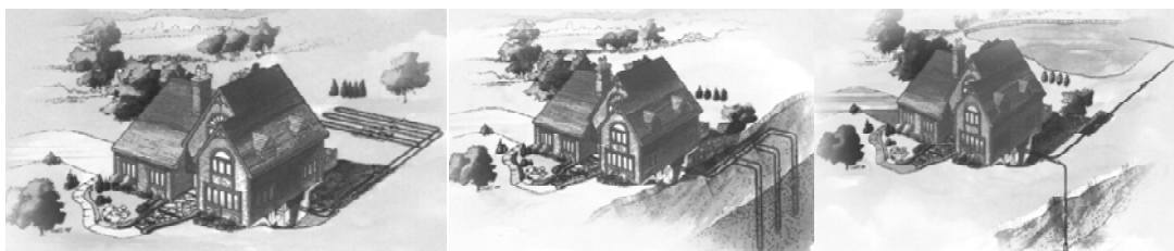
Figure 4.5 Ground source collectors a) horizontal standard, b) horizontal 'slinky' c) vertical (AIEA, 2006)
